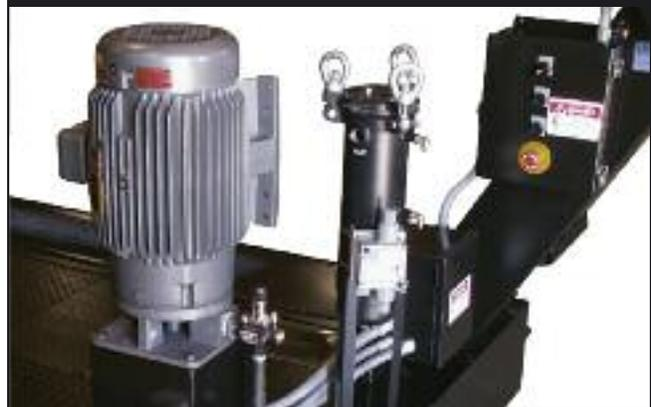
Heavy-duty pumps recycle coolant reliably. Automatic on-off float switches can be provided on request. Hennig can provide a complete coolant filtration solution.
