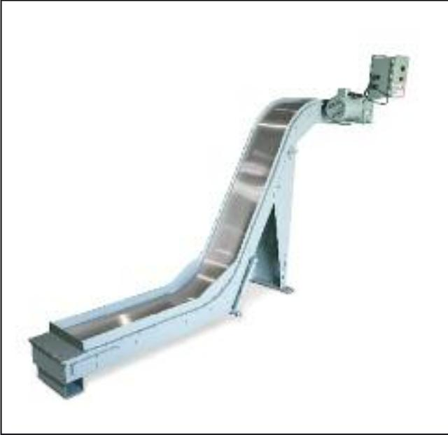
Magnetic chip conveyors are intended for ferrous material applications with small chips. The chips fall onto the conveyor's stainless steel surface and are conveyed by powerful magnets moving underneath. The chips are released from the magnets at the discharge end, and fall freely into a collection container.
