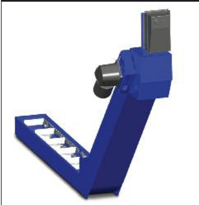
Scraper-type chip conveyors are most often used for cast iron, bronze or brass machining, which produces smaller chips that can nest together. Chips fall directly to the bottom of the conveyor, and scrapers drag debris to the discharge end of the conveyor.
