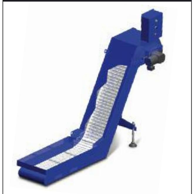
Hinge-belt chip conveyors, the most common format, offer an effective means of managing heavy chip loads and stringy chips. Chips that fall from the machine tool land on the conveyor belt and are conveyed away from the machine tool's precision surfaces.
